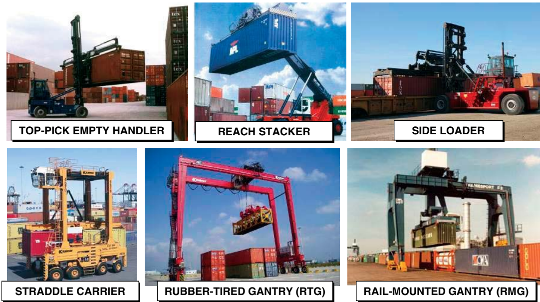
Figure 2–1. Container yard handling equipment types.
